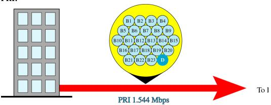
$64 \times 23 \text{ (B1-B23)} + 64 \text{ (D)} + 8 \text{ (overhead)} = 1.544 \text{ Mbps}$
